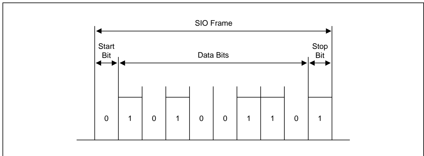
Figure 10-14. Serial I/O Frame Timing Diagram (Normal UART)
