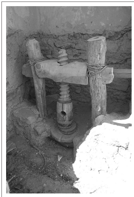
Fig. 1.12. Rigid frame direct-pressure screw press from the Monastery of St Anthony in Egypt
